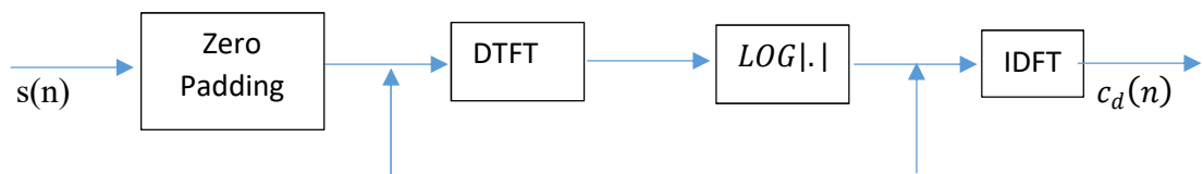
FIGURE 5.2: Computation of the real cepstrum using the DFT (After: [Deller, Proakis, Hansen, 1993]).
